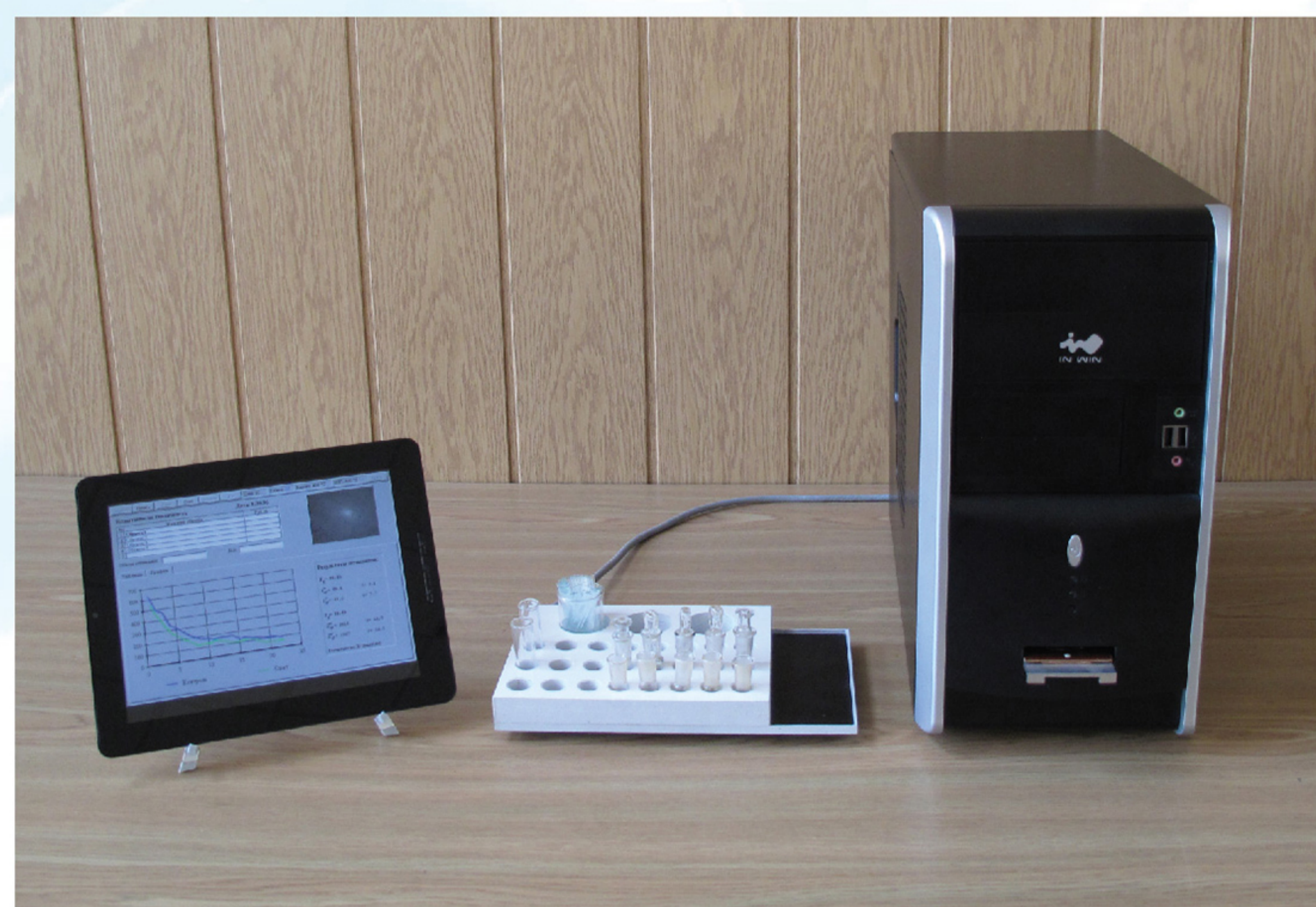
Fig. 1. Videoimage cytotoxicity analyzer
